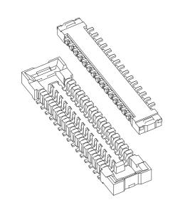
This is space saving type board-to-board connector with 0.4mm pitch, 0.8mm between PC boards and 2.0mm product width. 1.0mm Between PC boards is available by using dedicated receptacle.
